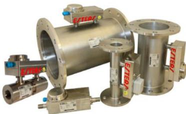
The dynamic range is 1: 100. The sensor responds very fast, T90 is below 50 ms. The medium pressure can be up to 40 bar, the maximum temperature is 120 ° C (for the ATEX version it is limited to 85 ° C). Repeatability is 0.1%, V4 steel construction guarantees corrosion resistance.
