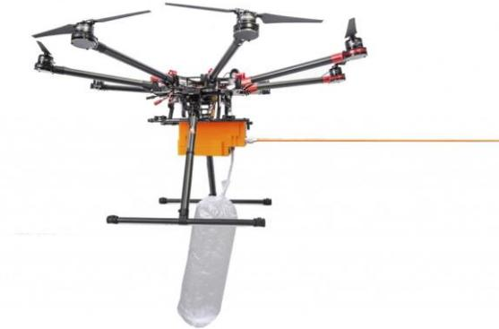
The Scentroid DR1000 can be used to sample and analyze ambient air at heights of up to 150 meters above ground level that was previously impossible to accomplish. Air quality mapping, model verification, analysis of potentially dangerous sites are all made possible by this novel innovation.
