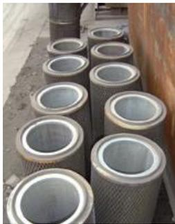
Over a period of time, Predict has helped to highlight a further problem with the filter. It was noted that gross filter deterioration was always apparent in the same two rows and as a result of this, the gas stream inlet to the filter was modified resulting in more even wear and extended filter life.
