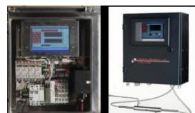
H<sub>2</sub>S and Sulphure analysers for gases and gasoline
